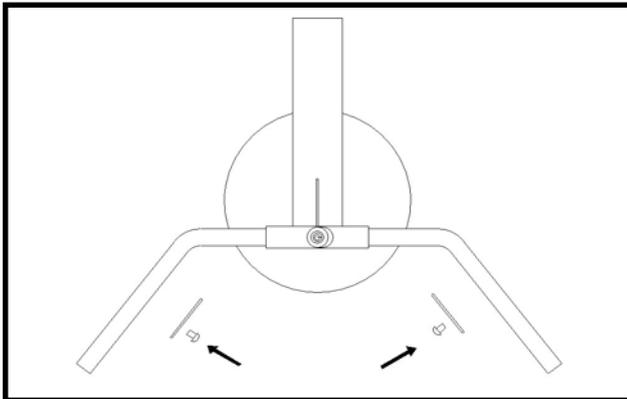
5. To Un-Lock Clamp: Insert key, rotate ½ turn, and pull on key until lock opens.
