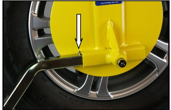
2. Fit left hand arm into channel until roll pin touches channel as shown. **(ARROW ON PICTURE)**
