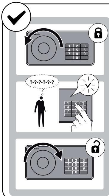
GB Check that your PIN code has been retained. Operate the lock three times without closing the door. If not, reset your PIN code.
