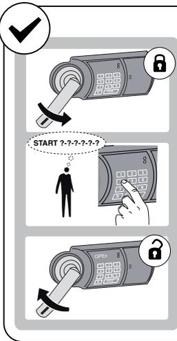
GB To check that your PIN code has been accepted operate the lock three times without closing the door. If unsure repeat the steps above.
