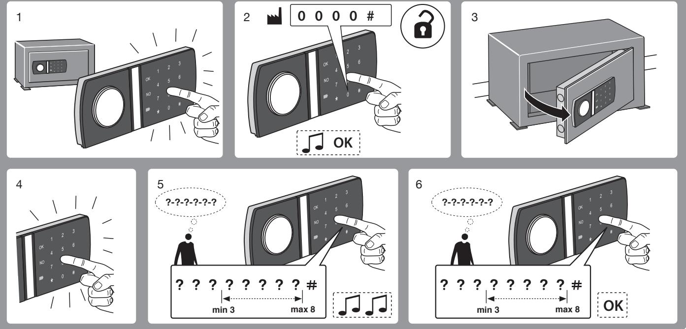
To check that your PIN code has been accepted operate the lock three times without closing the door. If unsure repeat the steps above.
