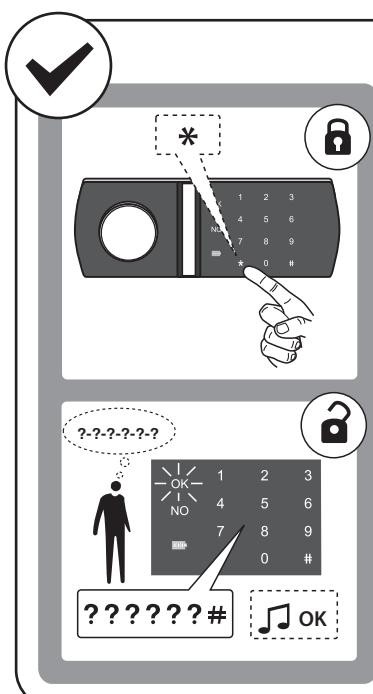
GB To check that your PIN code has been accepted operate the lock three times without closing the door. If unsure repeat the steps above.
