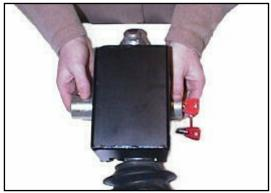
**6.** Push cup over end of locking bolt. turn key quarter turn clockwise to lock and remove key. Fit red plastic cover.
