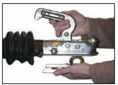
Insert dummy ring plate. If hitch handle is in raised position the plate can be used to release handle.
