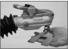
1. Insert dummy ring plate when trailer is unhitched by offering up at an angle and twisting into place.
