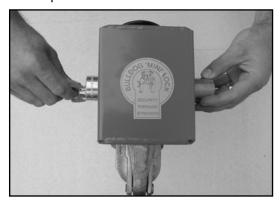
4. Insert Bulldog Super Lock Bolt through holes and put cup over the end. Turn key quarter turn clockwise to lock and remove key.
