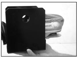
2. Offer up bottom channel according to your hitch type. Short fill strip at front for 12 - 14304 or tall fill in strip at front for standard hitch head.
