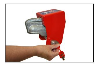
3. With the lock bolt in the unlocked position, insert it through both the holes of the cover. Fit the cup over the end of the lock bolt, then turn the key a quarter turn clockwise and remove.
