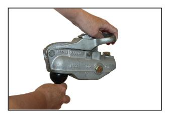
**1**. Insert the dummy ball when the trailer is unhitched by lifting the handle upwards and coupling in the normal way.
